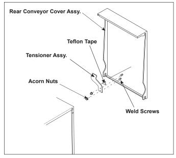
Figure 9. Replacing Spring Tensioner Assy.
